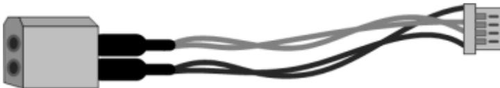
The right side of this cable goes into the Air Unit power port.
